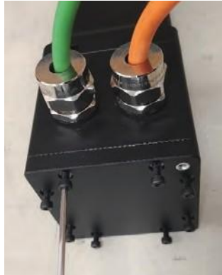
Figure 20: Loosen the rear cover screw
